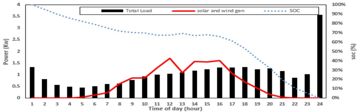
Fig. 3 Solar PV, Wind generation and battery Soc in summer (a) without DR, (b) with DR
