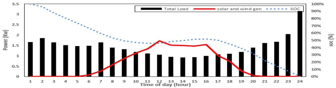
Fig. 6 Solar PV, Wind generation and battery Soc in spring (a) without DR, (b) with DR
