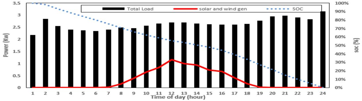
Fig. 4 Solar PV, Wind generation and battery Soc in fall (a) without DR, (b) with DR
